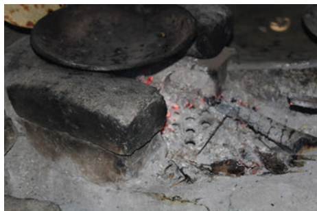
FIG. 2. The Mewar Angithi, a simple metal grate insert, is designed to improve airflow to flames to improve combustion efficiency and reduce wood usage, cooking times, and particulate emissions.
