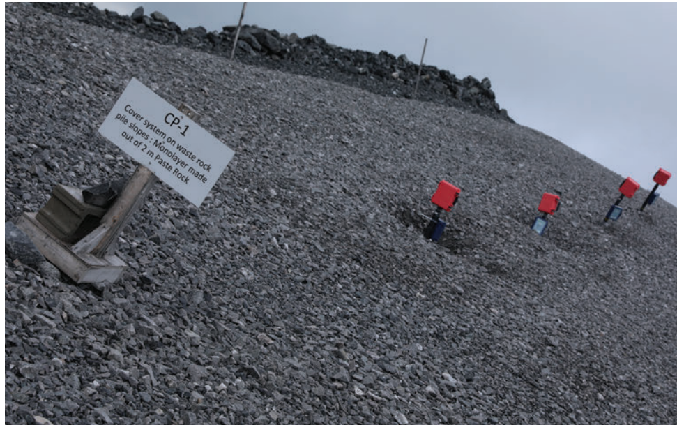
Sensors in the waste rock retention testing grounds.
